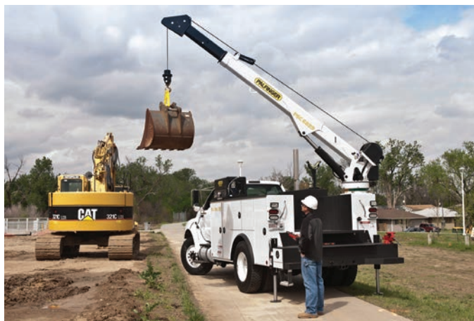
Any telescoping service truck crane with lifting capacity within 2,000 to 14,000 pounds falls within the rules of the OSHA 1926 Subpart CC.
